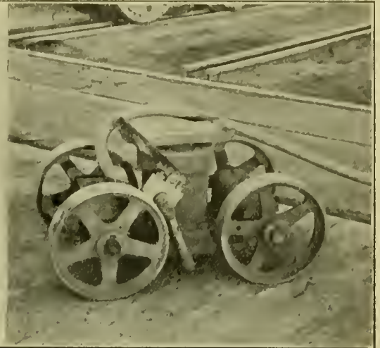
FIG. 21.—PORTABLE PNEUMATIC DEVICE FOR TURNING MOUNTED WHEELS.
